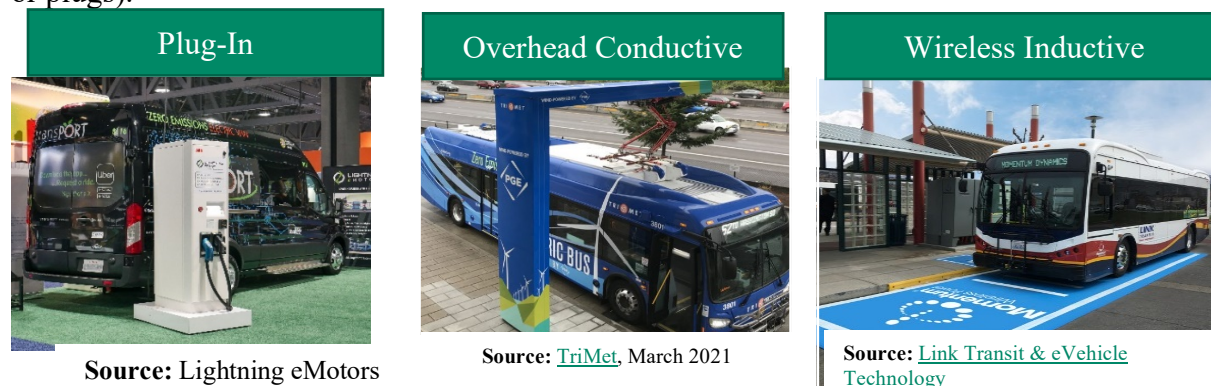
Figure 2: BEB Charging Infrastructure
